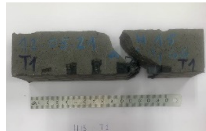
Fig. 2: An example of a broken reinforced concrete specimen.
