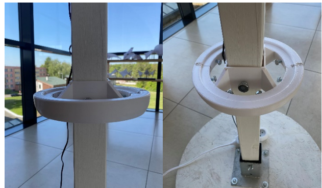
Fig. 2: Prototype of joint of the membrane to the support element made using 3D printing in scale approx. 1:4.
