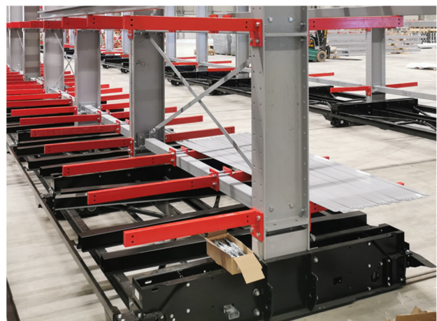
Fig. 2: Chassis part with connection to the rack building.
